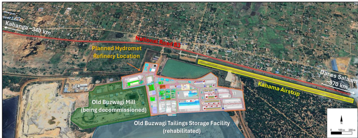
Figure 3: Satellite map with the 3D Model of the proposed Hydromet refinery superimposed, located at the site of Barrick Gold’s past-producing Buzwagi gold mine, Kahama, Tanzania. Phase 1 shown in color and Phase 2 in white.
