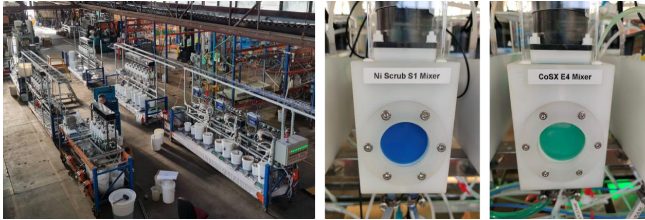
Figure 2: Semi-continuous pilot refinery test work underway at Lifezone’s Simulus Laboratory (left); close ups of solvent extraction (“SX”; center and right).
